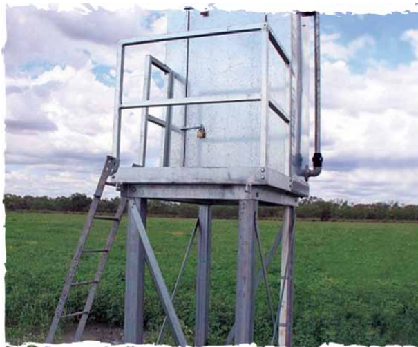
This gauging station in Narran Lake Nature Reserve records rainfall, water quality and air and water temperature and was funded through the Rivers Environmental Restoration Program. Photo: Peter Terrill, OEH
